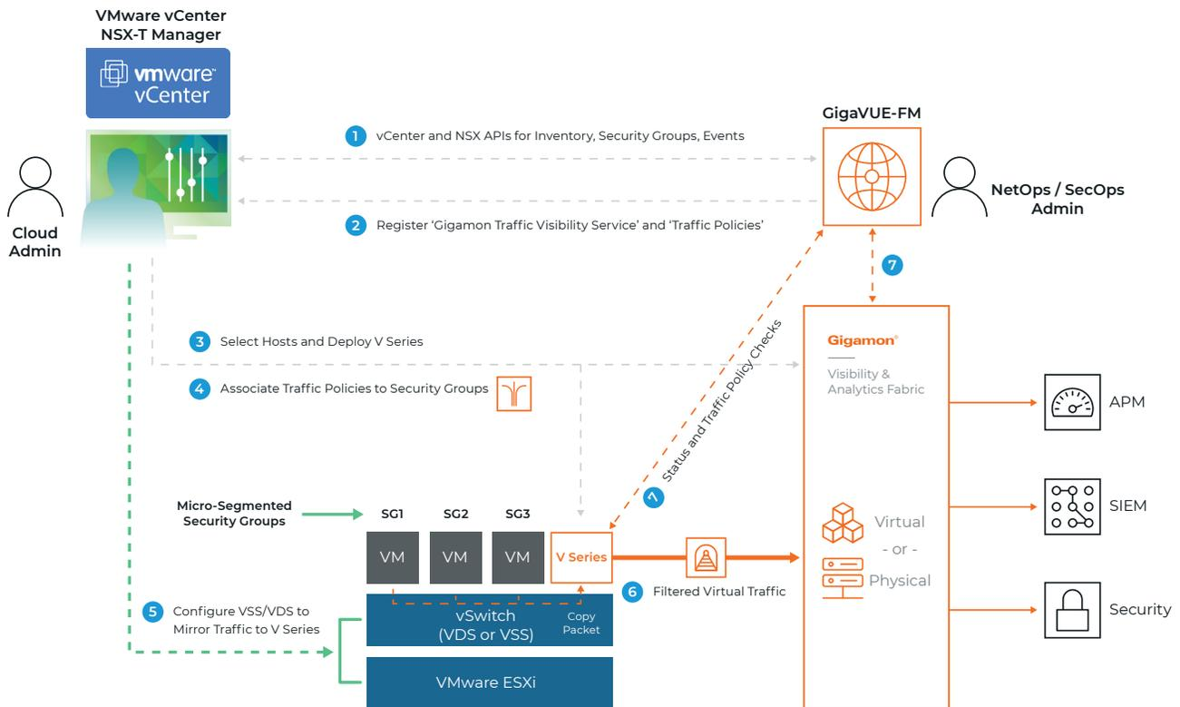
Figure 3. Straightforward seven-step process for provisioning, configuration and monitoring.
